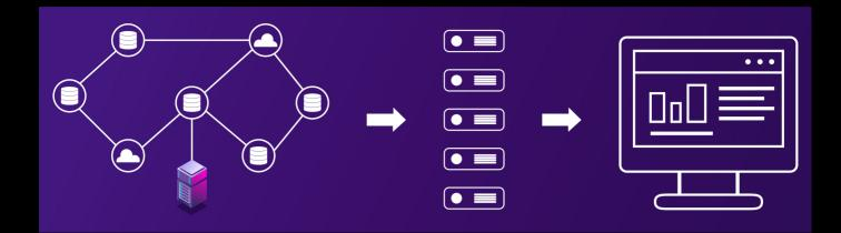
DNAfabric is powered by a wide area, clustered architecture. A scalable centralized controller provides management, metadata and analytics services while wide area data managers provide data visibility and data mobility services. DNAfabric components can be deployed across bare metal, virtual on-premise or cloud instances.
